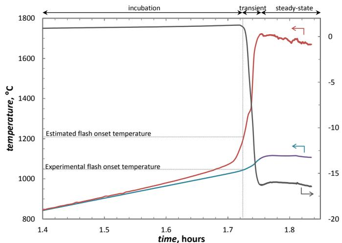
Furnace (blue) and estimated sample temperature (red) during shrinkage of a flash sintered 8YS sample.
